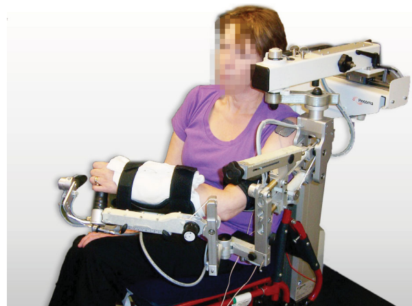
Fig. 1. Stroke patient using SAIL system: mechanical support device.
